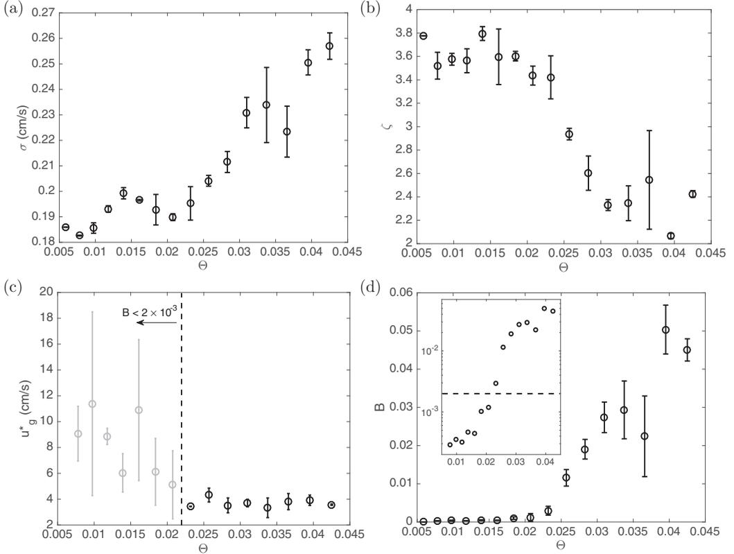
FIG. 7. Fit parameters (a)  $\sigma$ , (b)  $\zeta$ , (c)  $u_g^*$ , and (d)  $B$  from Eq. (3) as a function of Shields number  $\Theta$ . In all cases, the error bars are the standard error computed over six different experimental trials. We mark in (c) points (in gray) at which  $B < 2 \times 10^{-3}$ , where our fit for  $u_g^*$  is no longer physically meaningful. The inset to (d) shows the same data plotted on semilogarithmic axes, with a horizontal line at  $B = 2 \times 10^{-3}$ .
