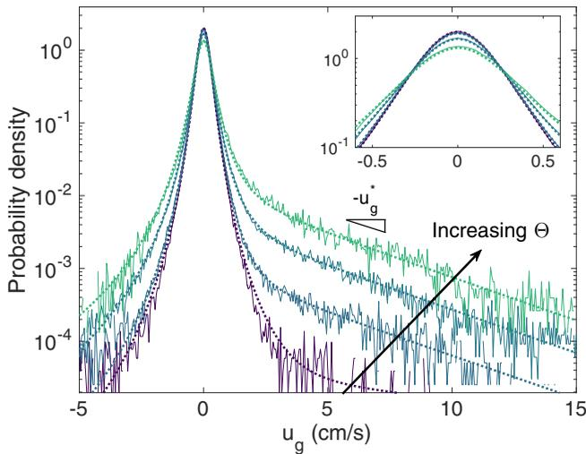
FIG. 6. The PDFs  $P(u_g)$  of grain velocities  $u_g$  (solid curves), for  $\Theta = 0.0059, 0.0232, 0.0283,$  and  $0.0425$ . Dashed curves show fits of the data to Eq. (3). The inset shows a close-up of the same data near the core of the PDF.
