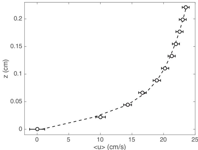
FIG. 2. Typical fluid velocity profile, as measured from the streamwise velocities  $u$  of tracer particles in the fluid. Each data point (open circles) represents a time average over all tracer particle trajectories for binned values of the height. The error bars show the standard deviation of the velocities in each bin. The dashed line is a fit following the procedure described by Rodríguez-López *et al.* [26], from which we extract the wall shear stress  $\tau_{\text{wall}}$  (see the text).
